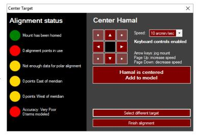
After one alignment star your CGX is minimally aligned. We recommend aligning to at least 4 stars for better goto accuracy, or ideally until all fields in the Alignment Status Window turn green.
