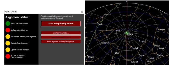
4. Click "Start new pointing model", then select a star in the Sky Viewer and click "Go to target". Or, you can choose from the Suggested Targets pulldown menu, which is broken up into the brightest objects in each quadrant of the sky. The telescope will slew to the area of that star and the Center Target screen will appear.
